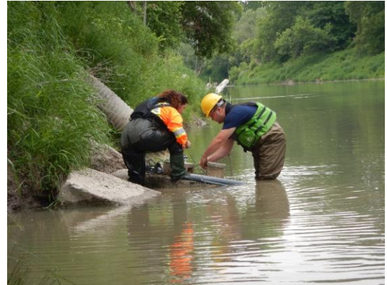
Figure 3: Madison McKnight and Randy Kirby prepare a PME miniDOT Oxygen logger for sampling dissolved oxygen and temperature conditions in the Thames River.
